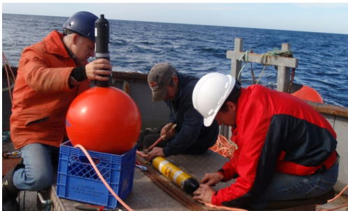
OTN technicians make final preparations to the mooring prior to deployment.
