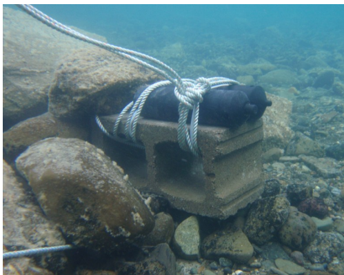
Mooring design of paired 69-kHz and 180-kHz VR2Ws in the Chilko River, BC. Photo by Matt Casselman.
