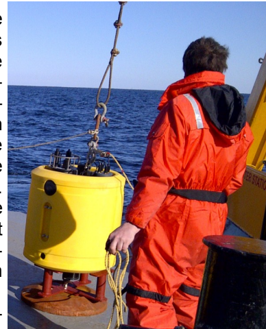
Benthic pod aboard Dominion Victory ready for deployment.
