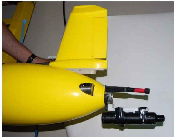
A Slocum Glider equipped with a Vemco acoustic receiver as part of tests of mobile tracking platforms.
